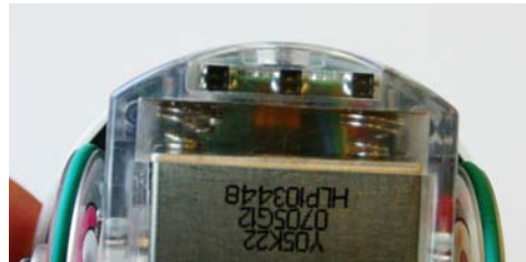
Figure 1.3 Three active IR sensor elements, Vishay's TCNT1000 are spaced out along a horizontal line
